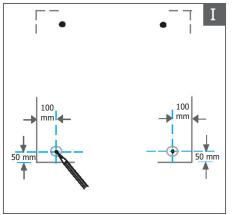
Mark drill positions for bottom fixing as indicated.
