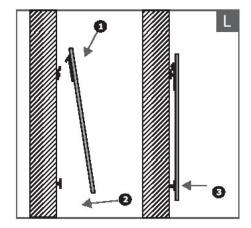
Hang object and push firmly at bottom end to attach bottom fixings to your object.
