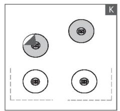
Remove protecting paper and aline buttons with marked edges.
