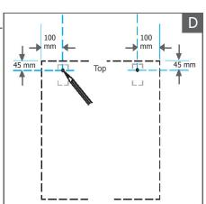
Position and mark drillpositions for top end as indicated.
