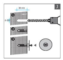
Drill 6 mm holes (38 mm deep) and fix with plugs and screws with round button facing the wall.
