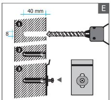
Drill 8 mm holes and fix mountingplates (with washer on the outside) with plugs and screws.
